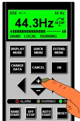
The VFD must be able to Change the Reference, Hz.
