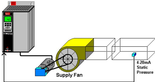
This lesson covers the basic functions of a Variable Frequency Drive (VFD) as it applies to fans.
