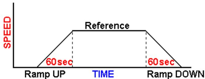
All ramp times are based on motor speed, 60Hz in Western Hemisphere, 50Hz in the Eastern Hemisphere.
