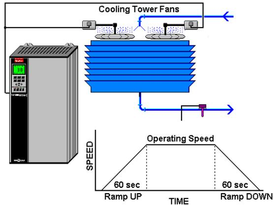
To reduce mechanical wear, it is important to control the acceleration, ramp up and deceleration, ramp down.
