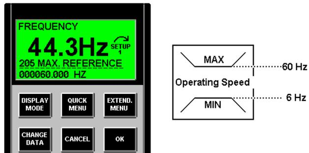
Limits on current, torque, speed, heat and voltage and others protect the VFD & motor.
