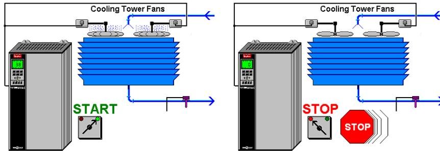
The VFD must be able to **START** and **STOP** the cooling tower fans.
