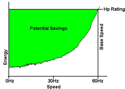
The most important function for the VFD with this fan application is to save energy.
