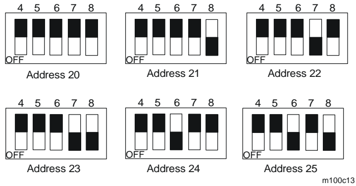
Figure 3: AHU/UNT/VAV Zone Bus Address Switch Settings
