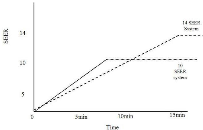
Multi capacity systems (such as our 20i dual compressor or 16i unloading scroll) allow for some cushion in the sizing calculations—but don't get carried away. Manuals J & S recommend that the system size is not more than 15% larger than the heat load calculation.
