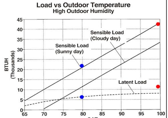
A properly sized multi stage system has just enough capacity to absorb the heat load in peak conditions, and reduces its capacity with milder outdoor temperatures. This modulating capacity allows for long run cycles throughout the day—maximizing comfort and minimizing the efficiency losses that are inherent in single stage systems.
